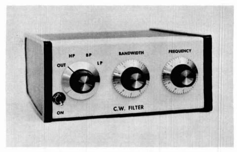
Tunable audio filter built by W1DTY is housed in Ten-Tec JW-5 enclosure. Input and output jacks are on rear panel.
